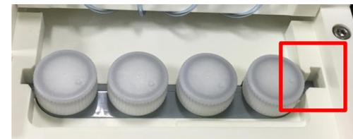
✘ L-shaped connector of the cartridge should follow the L-shaped guiding groove inside the instrument.
