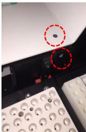
4. Push the sample plate holder to the right and remove the fixture.
