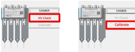
※ The storage and transportation condition may influence the gel-matrix and cause unstable current. If the current (gray line) is unstable during HV check, please repeat this step 2-3 times.
