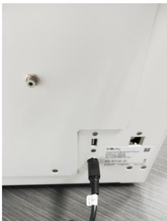
3. Plug the other side of the air tube into Qsep<sub>400</sub>
