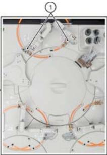
1. Sample probe wash solution set position
