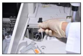
**6** Remove the lamp by turning the lamp holder counterclockwise, then pulling the lamp from the lamp receptacle. Handle the lamp by the lead wires.
