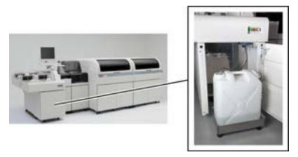
Figure 1.26 Master Wash Solution Tank
