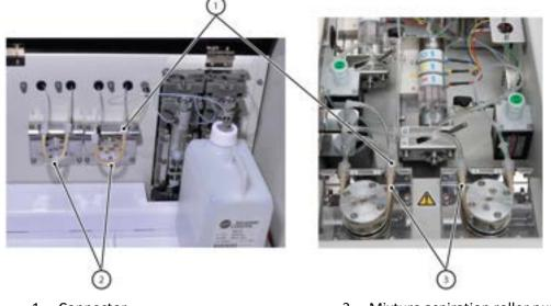
Figure 6.113 Mixture Aspiration and MID Standard Roller Pump Tubing
