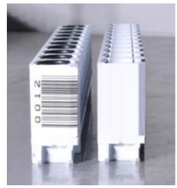
**2** Attach a new rack ID label on the rack. Place the label on the beveled edge of the rack with the numbers on the left (when looking at the rack).
