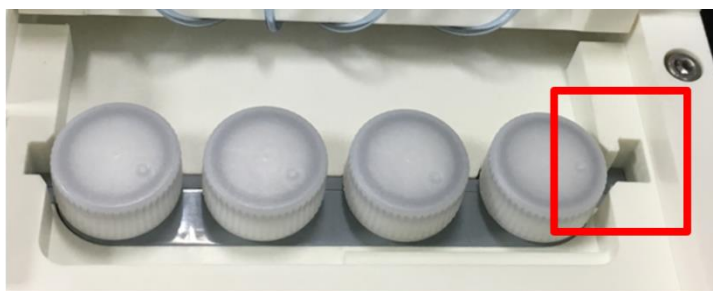
Figure 16 The L-shaped connector of the cartridge shall follow the L-shaped guiding groove
