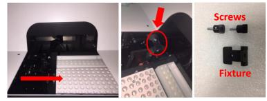
\*\*Before moving the instrument, the sample plate holder needs to be secured by the fixture to avoid system damage. Please keep the fixture and screws for later use.
