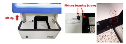
Push the sample plate holder to the right and remove the fixture.
