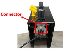
2. Plug the power cord into  $Qsep_{400}$ (Please make sure the label on the power cord is labeled  $Qsep_{400}$ ) 3. Plug the other side of the air tube into  $Qsep_{400}$
