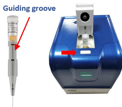
Figure 15 The guiding groove of the cartridge shall face the front
