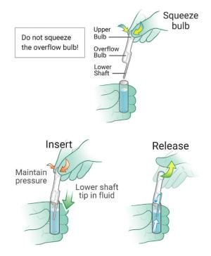
• The lower shaft should be full of liquid with no bubbles, and some fluid should be present in the overflow bulb.
