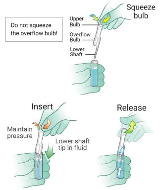
The lower shaft should be full of liquid with no bubbles, and some fluid should be present in the • overflow bulb.
