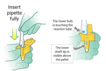
e. Firmly squeeze the upper bulb once, releasing the solution that is in the shaft. **None of the fluid will come out of the overflow bulb of the pipette.** It is normal for extra fluid to remain in the overflow bulb. **Do not squeeze** the overflow bulb of the pipette or reuse any leftover solution.
