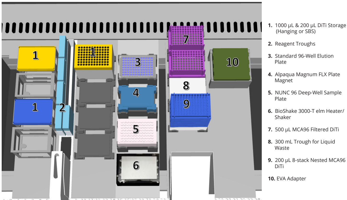
Figure 1. Tecan Fluent 780 deck layout for extraction of 96 blood samples with an input volume of 250 µL each.
